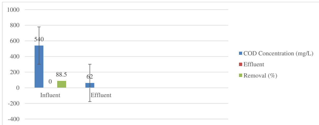
Figure 4.3.1 Comparative Analysis of Influent and Effluent COD Concentration
